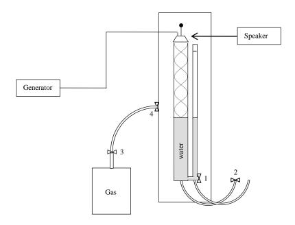
Fig. 1. Acoustic resonance measurement setup.
